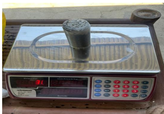
Figure 11. Measurement of Ceramic Media Mass using a Digital Weighing Scale prior to Capsule Assembly
