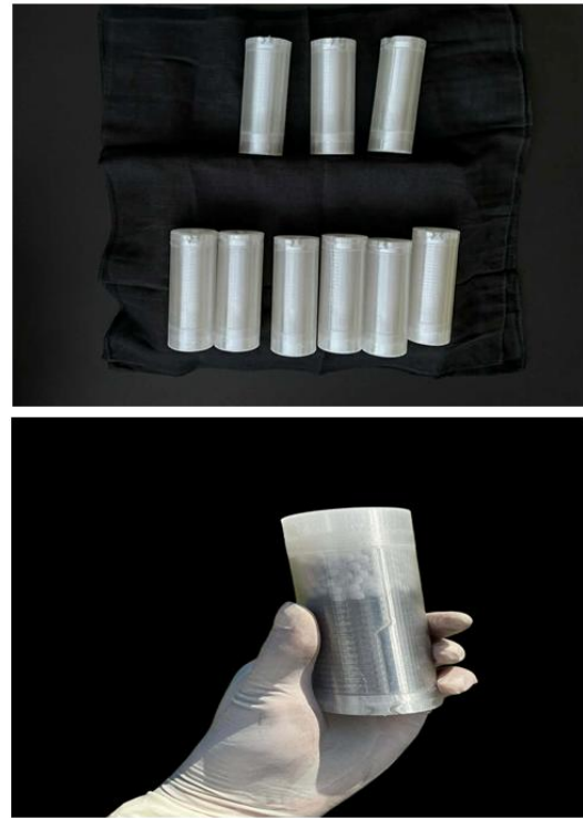
Figure 9. Developed Post-disinfection Capsule Showing Internal and External Components
