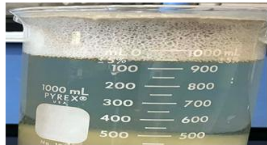
Figure 4.5 Formation of Visible Alum Floc after Flocculation
