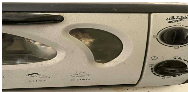
Figure 3.3 Oven-drying of YSPR at 130°C
