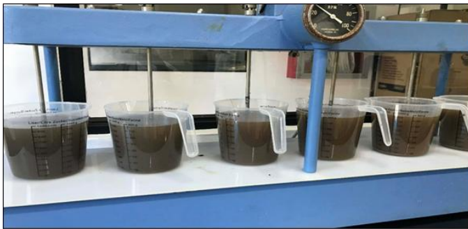
Figure 3.14 Jar Testing Setup – Trial 2 for 30 rpm Slow Mixing
