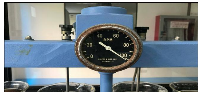
Figure 3.11 Jar Test Running at 100 rpm for Rapid Mixing
