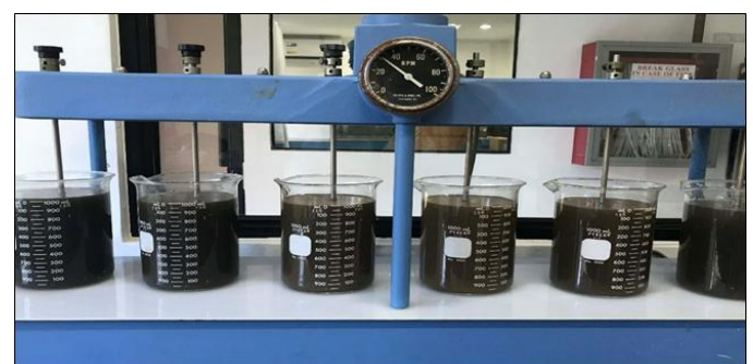
Figure 3.13 Jar Testing Setup – Trial 1 for 30 rpm Slow Mixing
