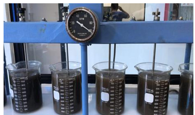
Figure 4.1 YSPR Treatment at 100 rpm for Rapid Mixing
