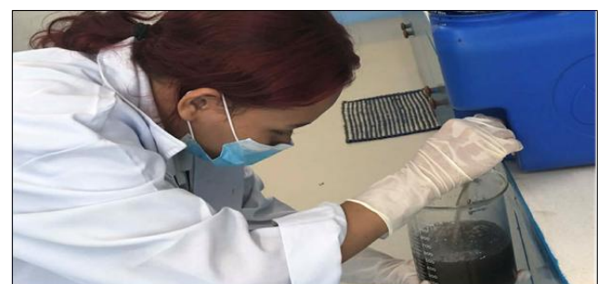
Figure 3.12 Jar Test Running at 30 rpm for Slow Mixing
