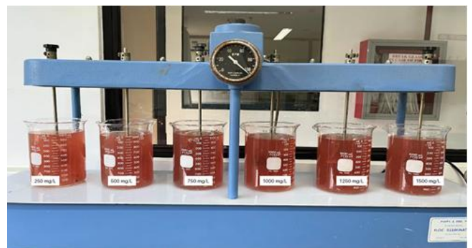
Figure 3.3. Using Jar Tester to Conduct the Coagulation of Different Dosages (Trial 1)
