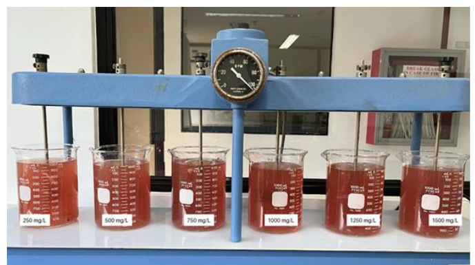
Figure 3.4. Using Jar Tester to Conduct the Coagulation of Different Dosages (Trial 2)
