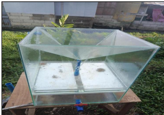
Fig. 2. Inverted-pyramid solar still undergoing the distillation process
