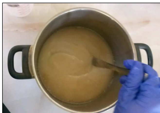
Figure 2.11. Appearance of 'trace' after thorough mixing
