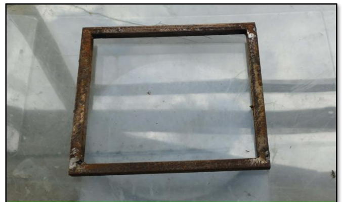
Fig. 2. Actual Steel Mold Utilized for Fiberboards Fabrication.
