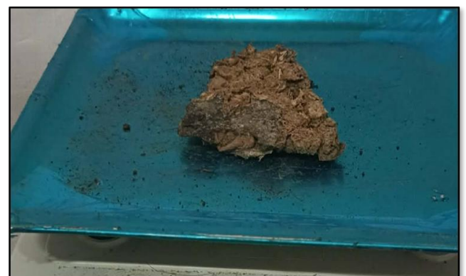
Fig. 5. Unearthed Eco-Fiberboards Week 2 (FB1).
