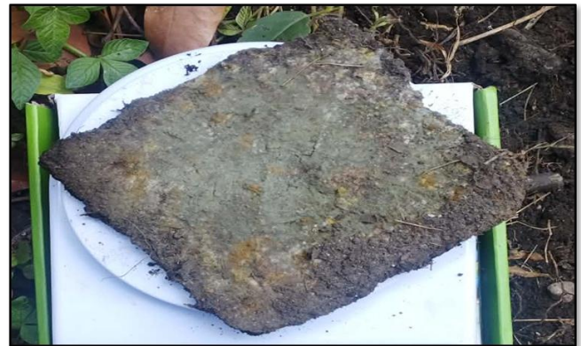
Fig. 4. Unearthed Eco-Fiberboards Week 1 (FB1).
