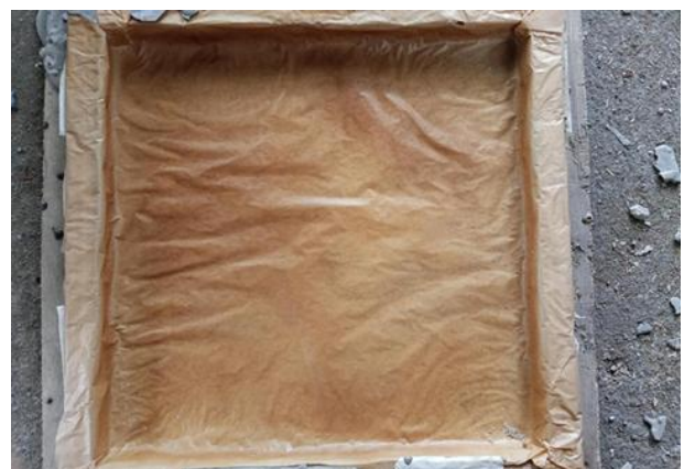
Figure 2.5. Insulation Panel Molder Used Shaping and Forming the Composite Panel
