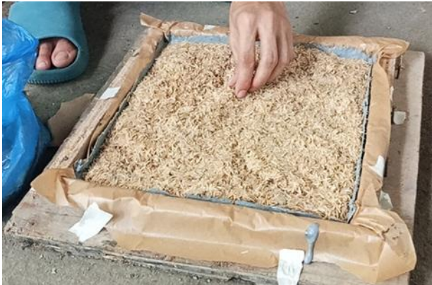
Figure 2.6. Photo Shows the Addition of the RH Core in the First Layer
