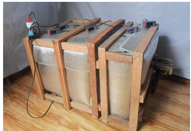
Figure 2.14. The Modified Thermal Conductivity Apparatus used to Measure the Thermal Conductivity of the Sandwich-Structured Insulation Panel
