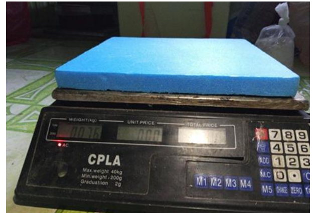
Figure 2.13. Weighing the XPS Insulation Using Digital Weighing Scale
