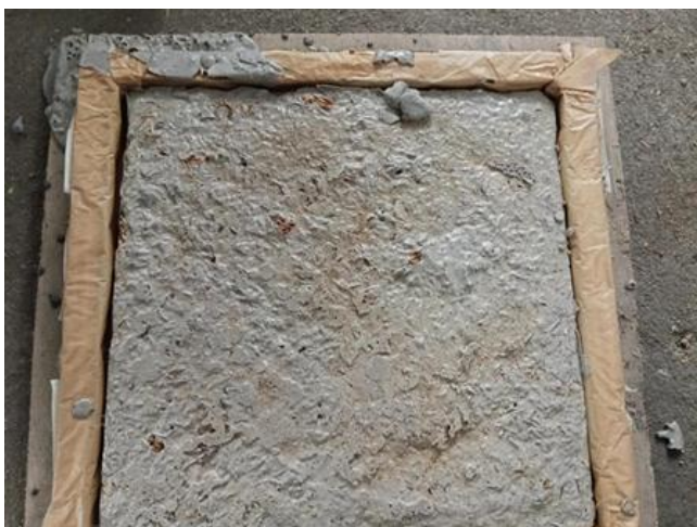
Figure 2.7. Photo Showing the Insulation Panel After Composite Blending and Layering Formation, Stabilize Through 1-2 Days of Passive Cooling
