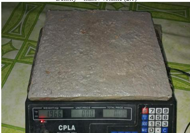
Figure 2.12. Weighing the Developed Insulation Panel During Digital Weighing Scale
