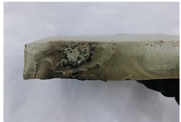
Figure 2.8. The Developed Insulation Panel after Subjected to Modified Ignitability Test
