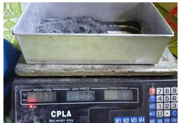
Figure 2.4. Weighing of RHA Using a Calibrated Digital Balance Prior to Mixing
