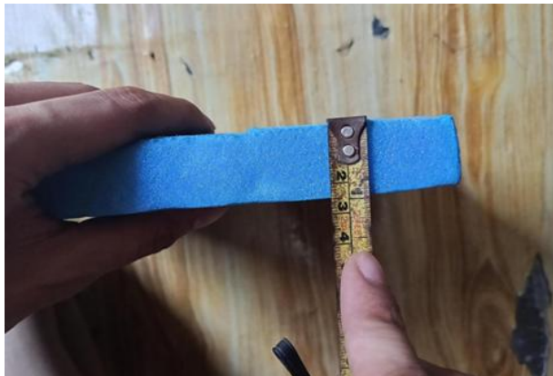
Figure 2.11. Measuring the Thickness of the XPS Insulation Panel Using Steel Tape
