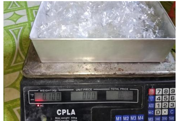
Figure 2.3. Weighing of the PET Plastic Using a Calibrated Digital Balance Prior to Processing
