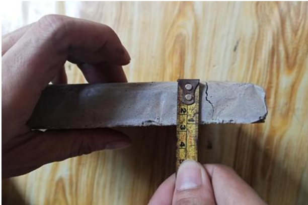
Figure 2.10. Measuring the Thickness of the Developed Insulation Panel Using Steel Tape
