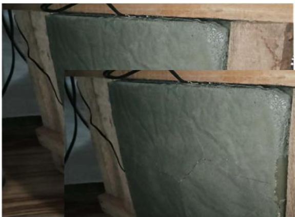
Figure 2.15. The Photo of XPS Insulation During the Modified Thermal Conductivity Test
