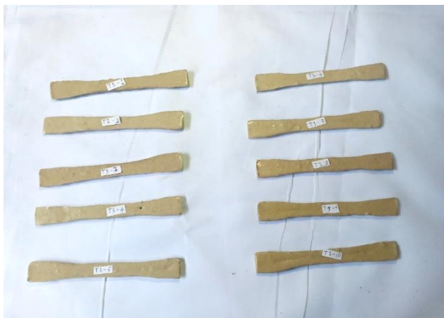
Figure 3.21. Treatment 0 Test Specimens for Tensile Strength ASTM D638
