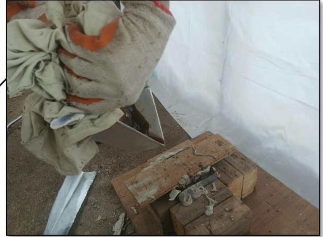
Figure 3.13. Garden Pot Undergoing Compaction
