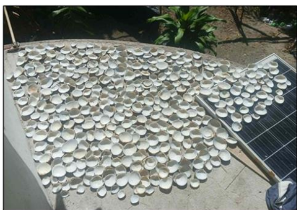
Figure 3.2. Discarded Clam Shells Undergoing Sun Drying Process
