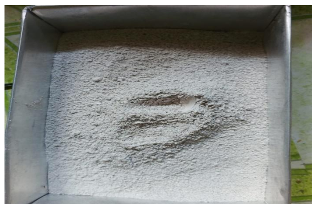
Figure 3.5. Powdered Clam Shells after Sieving
