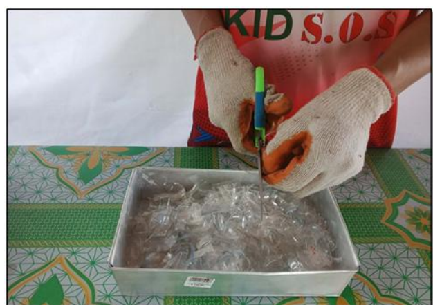
Figure 3.7. Cutting of PET Plastic Waste
