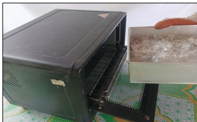
Figure 3.8. Placement of PET Plastic Waste in the Oven
