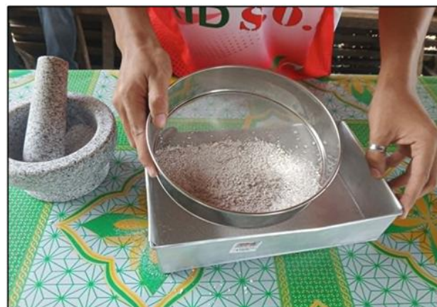
Figure 3.4. Sieving the Powdered Clam Shells Using Sieve No. 50 (0.30mm)
