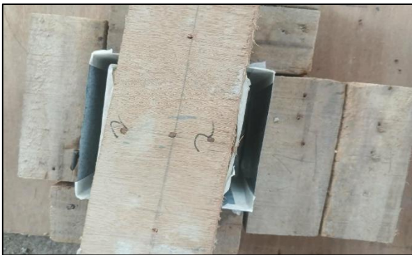
Figure 3.12. Top Mold Used in the Actual Experimental Setup
