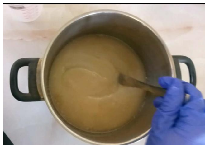
Figure 2.11. Appearance of 'trace' after thorough mixing
