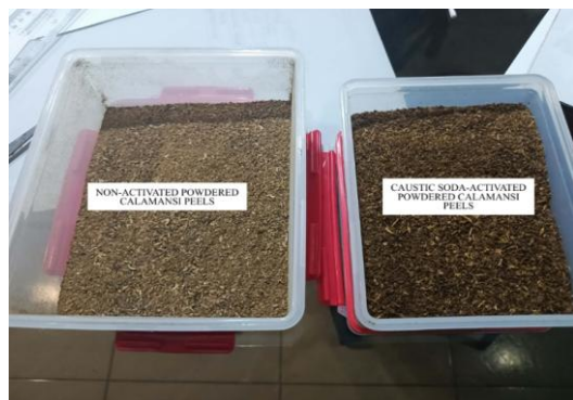
Fig. 4. Color Variation Between ACP and NACP Samples.
