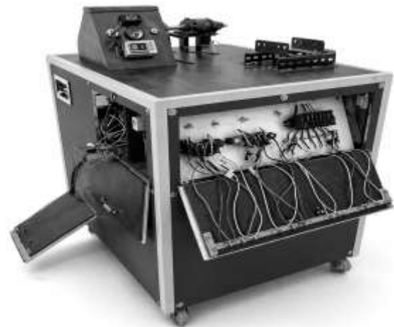
Figure 3. The Completed Automotive Charging System Trainer
