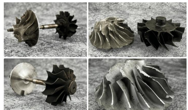
PLATE 4: Compressor and Turbine Blade Components Showing Tear and Wear
