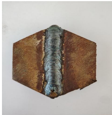
Fig. 4. Morphology of welding results at Porosity 0.1 %
