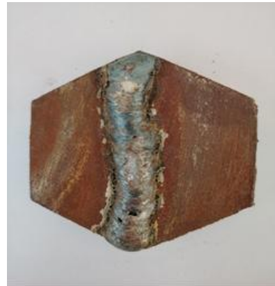
Fig. 3. Morphology of welding results at Porosity 1.2%
