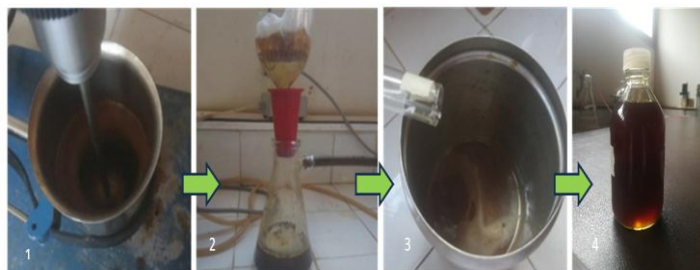
Fig. 3. Manufacturing process of the antihypertensive oral solution based on C. occidentalis root extract (1 : Homogenization ; 2 : Filtration ; 3 : Addition of excipients and preservatives ; 4 : Quality controls)
