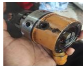
Fig. 7. Head pump rotor condition
