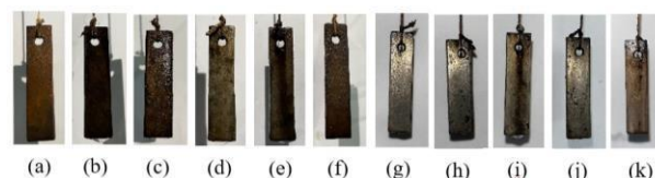
Macro Photographs of Kersen Leaf Extract Inhibitor on ASTM A53 Steel (a) 0 ppm; (b) 200 ppm; (c) 400 ppm; (d) 600 ppm; (e) 800 ppm; (f) 1000 ppm; (g) 1200 ppm; (h) 1400 ppm; (i) 1600 ppm; (j) 1800 ppm; (k) 2000 ppm.
