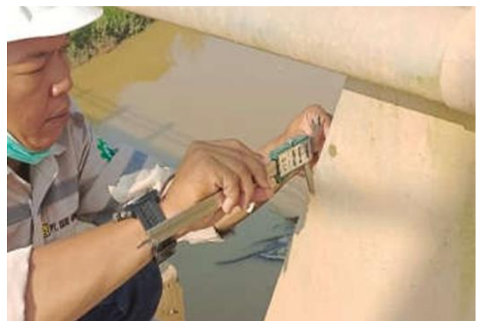
Fig. 5. Measurement of steel profile using sigmate.
