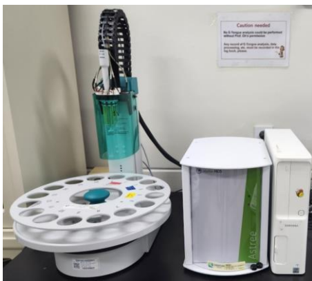
Fig. 1: Astree Electronic tongue
