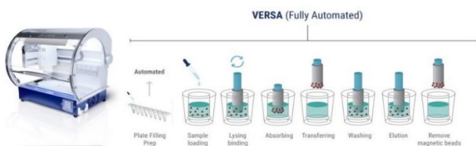
Fig. 5. Steps performed within the Automated DNA Extraction System [24]
