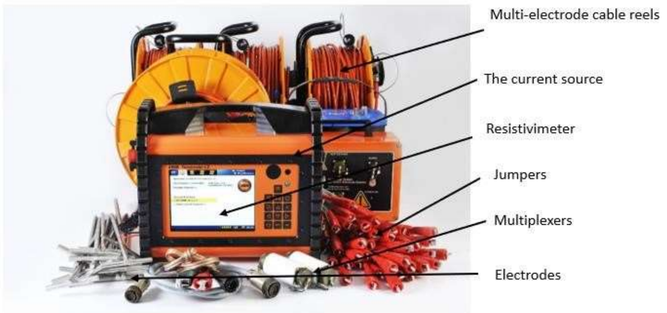
Figure 6. Geoelectric measurement equipment
