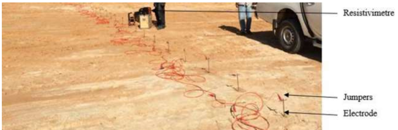
Figure 8. Example of a 2D tomography acquisition system
