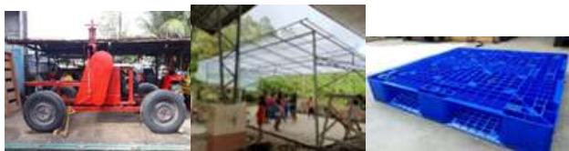
Fig. 3. Abaca stripping machine, all-weather dryer and pallet equipment in the processing center in North Cotabato, 2021
