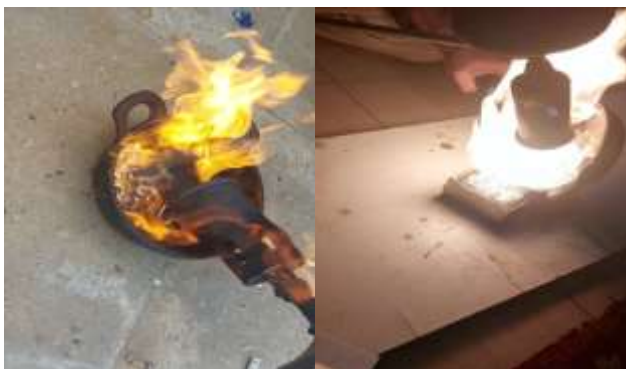
Figure 2: The Lead Melting on Reinforce Concrete
