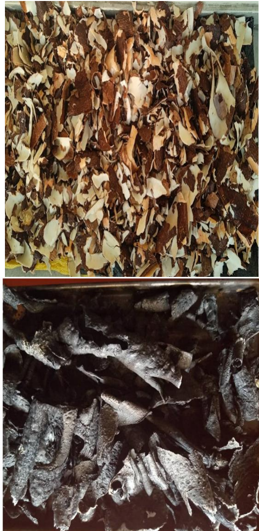
Figure 2: A; Freshly washed cassava peels, B; Cassava Peel Biochar produced from slow pyrolysis
