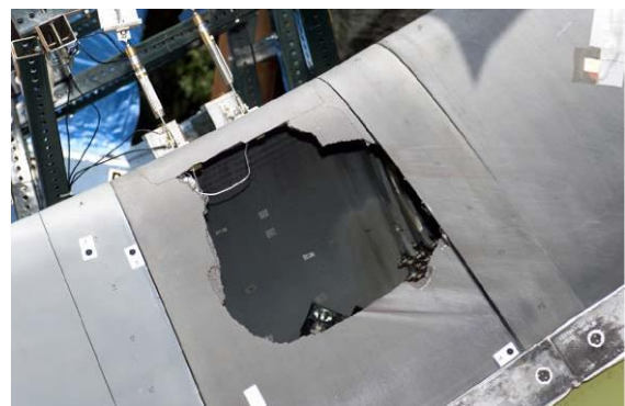
Figure 11. A mock-up of a space shuttle leading edge made with an RCC-panel taken from Discovery. Simulation of known and possible conditions of the foam impact on Columbia's final launch showed brittle failure of RCC Source: https://www.semanticscholar.org/paper/A-Summary-of-the-Space-Shuttle-Columbia-Tragedy-and-Melis-Carney/00b3e71009903e51302b8b4fbb719bbc667c8214 , Accessed: July 14, 2023.
