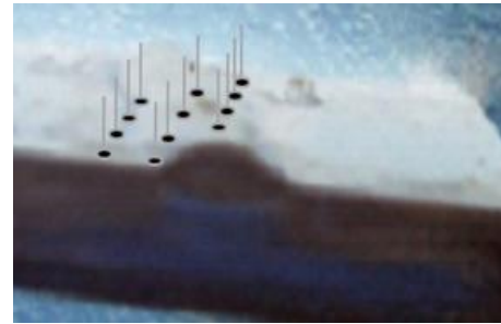
Fig. 3. Locations of test points of the hardness test samples. Base metal (BM), heat affected zone (HAZ), weld metal WM
