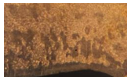
Fig. 5. Variation and defects in Microstructure of HAZ due to temperature difference.
