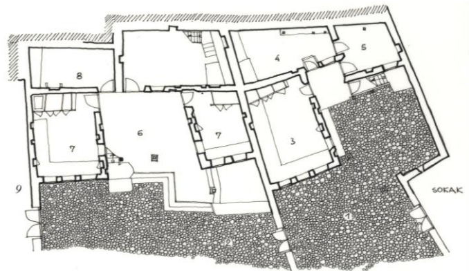
Figure 3. The Kajtaz family house in Mostar. Ground floor: 1. Men's courtyard, 2. Women's courtyard, 3. Men's halvat, 4. Mutvak, 5. Hudjera, 6. Hayat, 7. Women's halvat, 8. Mutvak, 9. Garden Source: A. Hadrovic (Drawing based on archival material of Stari Grad Mostar archive, 1984)
