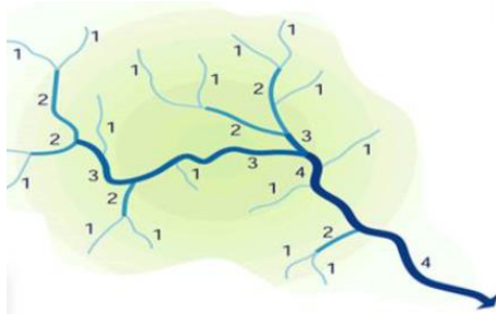
Fig. 2. Determination of the stream order using the Strahler method
