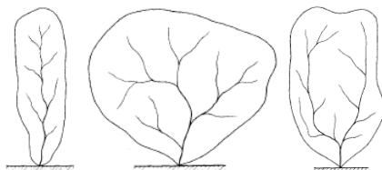
Fig. 3. Types of drainage shape; elongated shape (left), radial shape (center), and parallel shape (right)
