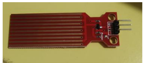
Fig. 5. Water level sensor module.
