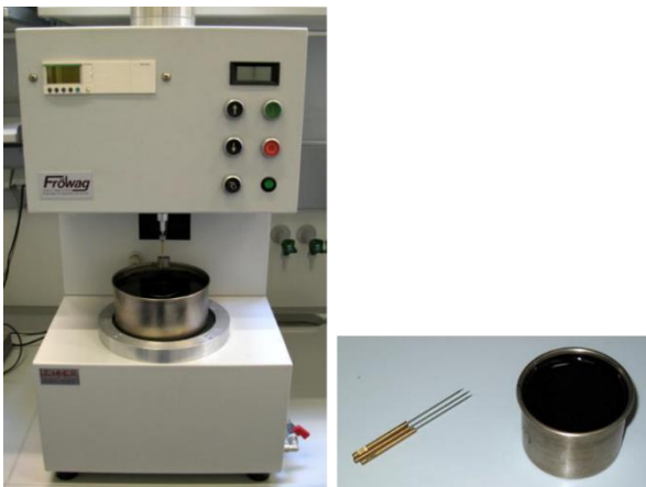
Figure 1: left: Apparatus for conducting the penetration test for bitumen, right: 100 g needle [2]
