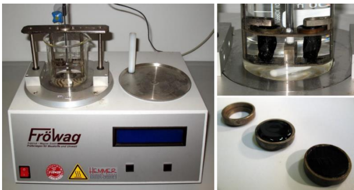
Figure 5: left: Ring and ball machine, top right: Bitumen bag, bottom right: Measuring rings [2]
