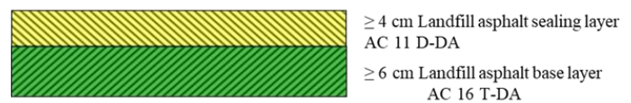
Fig. 3. Landfill asphalt sealing component consisting of a landfill asphalt base layer and a landfill asphalt sealing layer [13]
