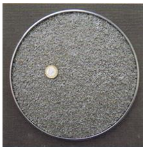
Figure 10 a) Henau Quarzit 2/4 is not only exceptionally bright, but also impresses with its high PSV value and rough surface. [7]
