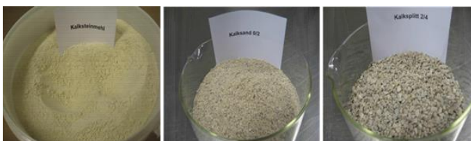
Figure 2. Composition of the mastic asphalt: lime flour (filler), lime sand 0/2 mm and lime chipping 2/4 mm [1, 6]
