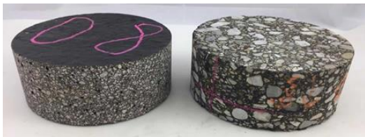
Figure 5. Mastic asphalt (left), rolled asphalt (right) [1]
