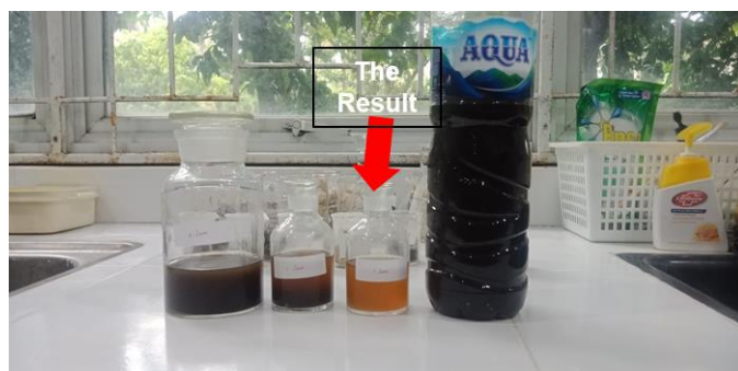
Fig. 7. The result of oil waste purification using bentonite from Cantayan Formation
