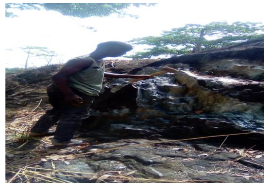
Fig. 3A. Quarrying by wedging method at Fonikoh forest edge Community
