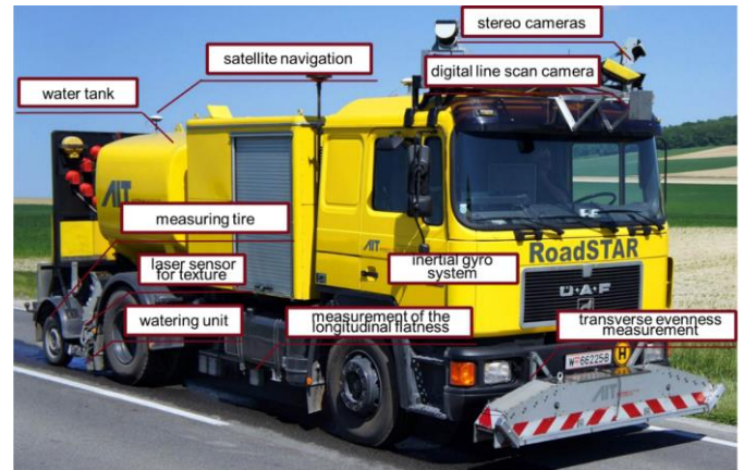
Fig. 12. The "RoadSTAR" system for measuring road skid resistance, road surface etc. [3, 14]
