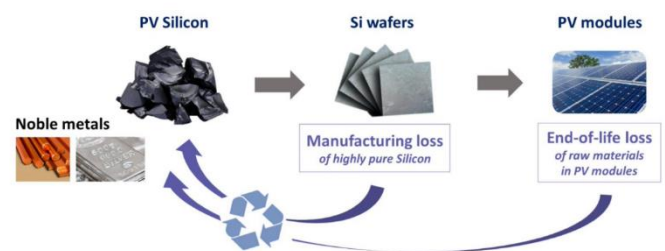
Fig. 1. Recuperation of ultra-pure silicon and other metals from solar panel's end of life Source: (ROSI – Return of Silicon, 2021)
