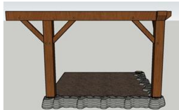
Fig. 7. Structure of dalem bale (teken and belandar)
