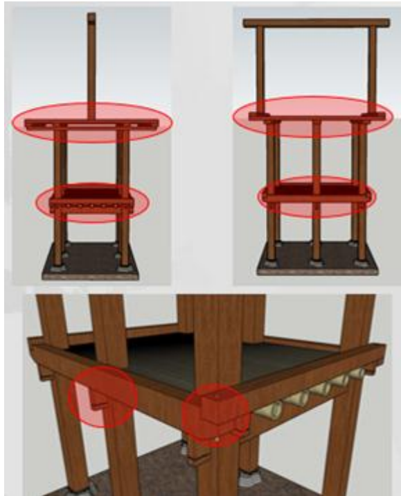
Fig. 10. Reinforced structure of inan bale
