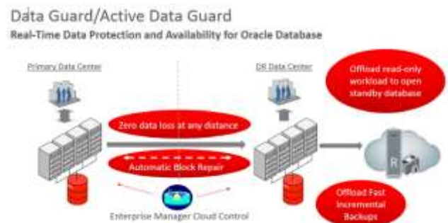
Fig. 3. Architecture of Oracle Active Data Guard
