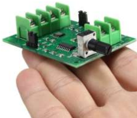
Figure 3. 5V-12V DC Brushless Motor Driver Board Controller For Hard Drive Motor
