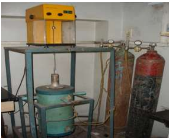
Fig. 4. Thermo gravimetric apparatus used for reduction.
