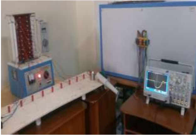
Fig. 6. Experimental setup of PFN, food chamber & DSO.
